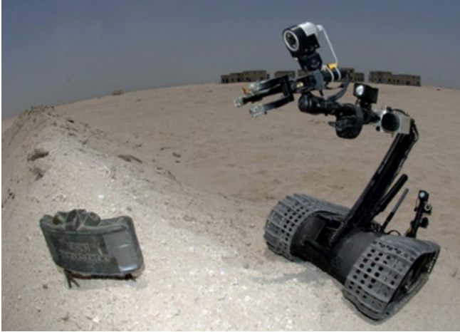
A Talon 3B robot approaching an anti-personnel mine during a training exercise in Iraq.
